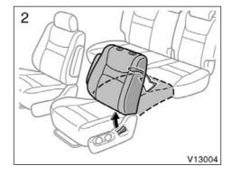
Pull the seatback angle adjusting lever to unlock and push down the seatback.
