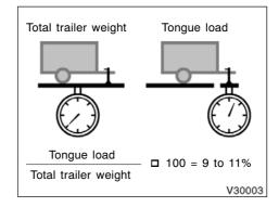
The trailer cargo load should be distributed so that the tongue load is 9 to 11% of the total trailer weight, not exceed the following.
