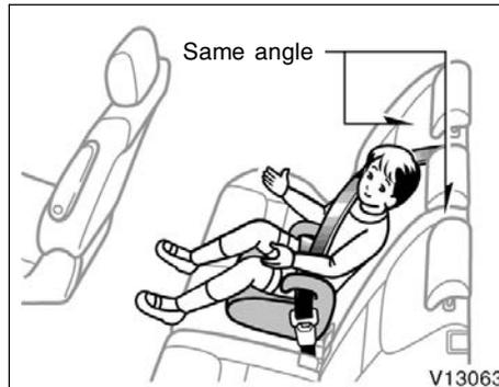
● When installing a child restraint system in the rear center position, align both seatbacks at the same angle. Otherwise, the child restraint system cannot be securely restrained and this may cause serious injuries in a collision.
