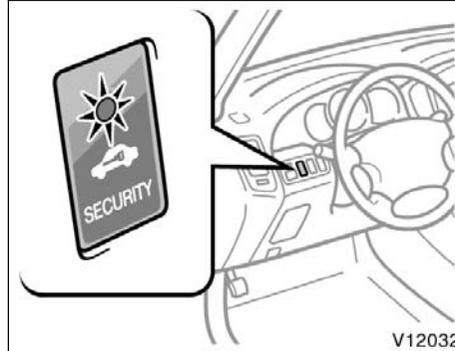
The system is automatically set when the key is removed from the ignition switch. The indicator light will start flashing to show the system is set.
