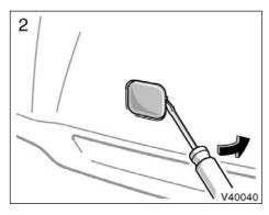
2. Remove the front towing eyelet cover on the front bumper.
