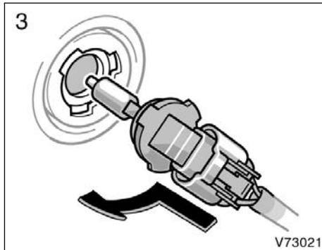
3. Insert the bulb base into the mounting hole by turning it clockwise.
