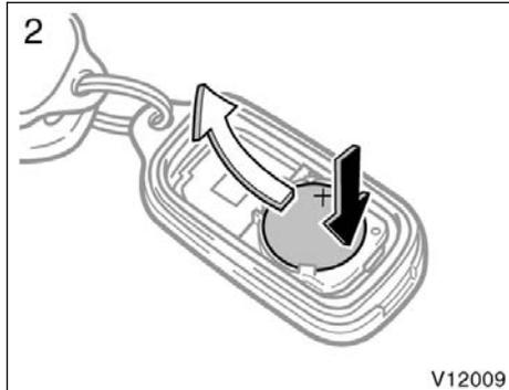
2. Remove the discharged transmitter battery.
