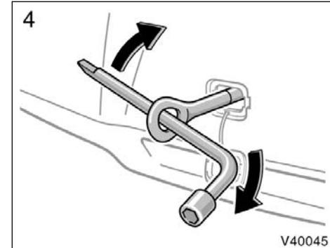
4. Tighten the front towing eyelet securely by a wheel nut wrench.
