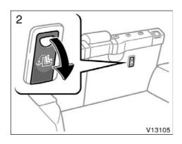
Open the anchor bracket cover with the symbol as shown in the illustration.
