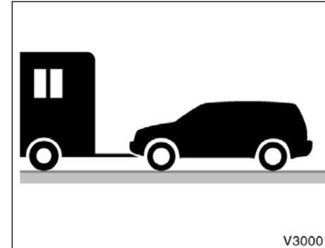
Your vehicle can be dinghy towed (with four wheels on the ground) from the front behind a motorhome.
