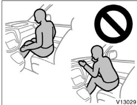
● Do not sit on the edge of the seat or lean over the dashboard when the vehicle is in use. The front airbags inflate with considerable speed and force; you may be killed or seriously injured. Sit up straight and well back in the seat, and always use your seat belt properly.
