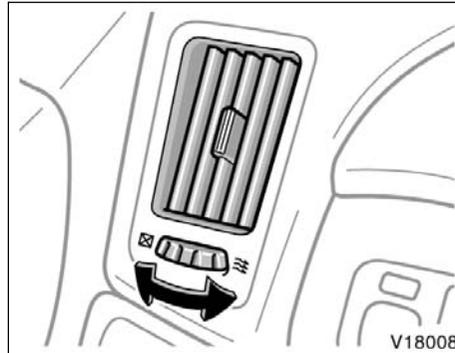
If air flow control is not satisfactory, check the side vents. The side vents may be opened or closed as shown.
