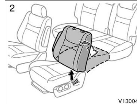
2. Pull the seatback angle adjusting lever to unlock and push down the seatback.
