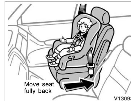
● A forward-facing child restraint system should be allowed to be put on the front passenger seat only when it is unavoidable. Always move the seat as far back as possible, because the force of the deploying front passenger airbag could cause death or serious injury to the child.
