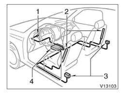
The SRS side airbag system consists mainly of the following components, and their locations are shown in the illustration.
