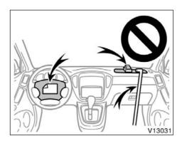
• Do not put objects or your pets on or in front of the dashboard or steering wheel pad that houses the front airbag system. They might restrict inflation or cause death or serious injury as they are projected rearward by the force of the deploying airbags. Likewise, the driver and front passenger should not hold things in their arms or on their knees.
