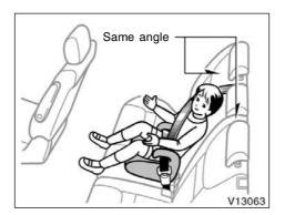
• When installing a child restraint system in the rear center position, align both seatbacks at the same angle. Otherwise, the child restraint system cannot be securely restrained and this may cause serious injuries in a collision.
