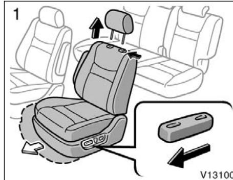
1. Remove the head restraint. Push the seat position adjusting switch forward to slide the seat further forward than the front-most lock position.
