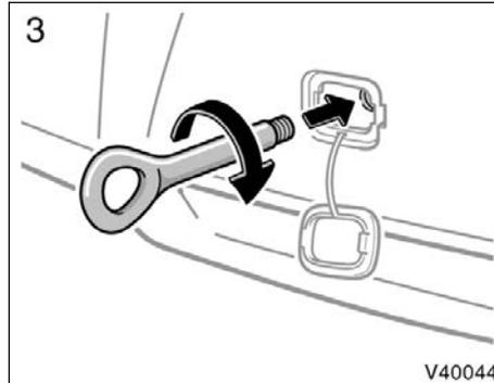
3. Secure it to the hole on the bumper by turning clockwise.
