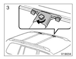
In order to fix the cross rails to the appropriate length, turn the upper knobs clockwise after tightening all of the side knobs.
