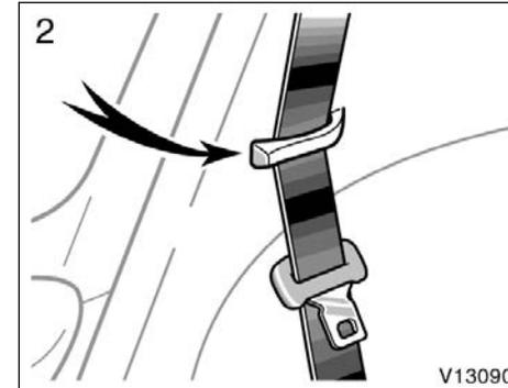
2. Make sure the outer seat belts passes through the hangers when folding the rear seat.
