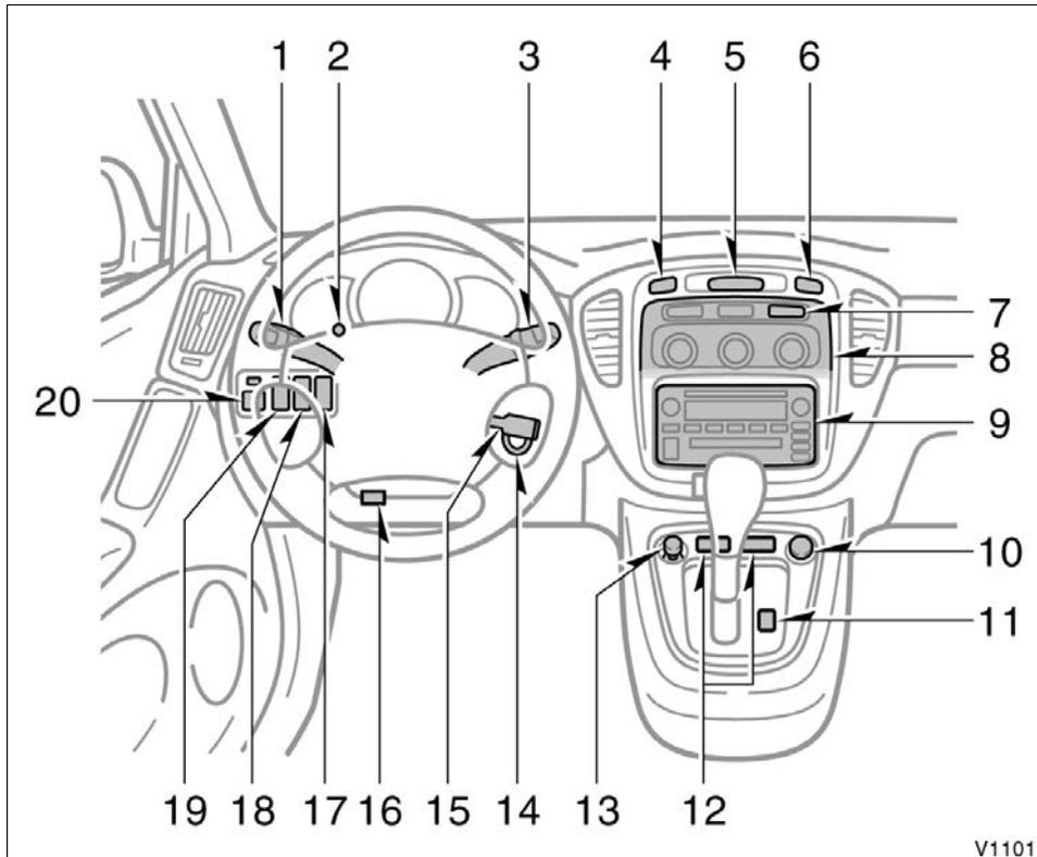
1. Headlight, turn signal and front fog light switches
