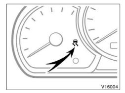
The vehicle skid control system helps integrated control of several systems such as an anti-lock brake system, brake assist system, traction control, engine control, etc. This system automatically controls the output of the brakes or engine to help prevent the vehicle from skidding when cornering on a slippery road surface or abrupt steering wheel operation occurs.
