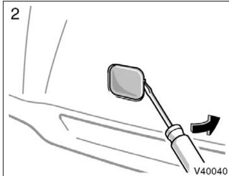
2. Remove the front towing eyelet cover on the front bumper.
