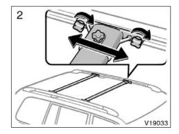
Slide the cross rails to the appropriate position for loading the luggages and turn the side knobs clockwise to tighten the cross rails securely.
