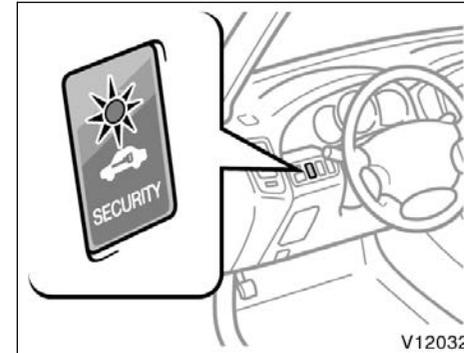
To deter the vehicle theft, the system is designed to give an alarm if any of the side doors, back door or hood is forcibly unlocked or the battery terminal is disconnected and then reconnected when the system is set.
