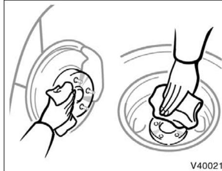
Before putting on wheels, remove any corrosion on the mounting surfaces with a wire brush or such. Installation of wheels without good metal-to-metal contact at the mounting surface can cause wheel nuts to loosen and eventually cause a wheel to come off while driving. Therefore after the first 1600 km (1000 miles), check to see that the wheel nuts are tight.
