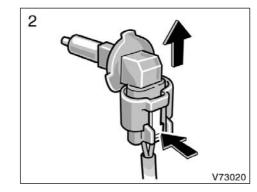
2. Pull the bulb out of the bulb base and install a new bulb.
