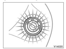
For easy access to the ignition switch, the ignition switch light comes on when any of the side doors are opened.
