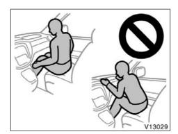
Do not sit on the edge of the seat or lean over the dashboard when the vehicle is in use. The front airbags inflate with considerable speed and force; you may be killed or seriously injured. Sit up straight and well back in the seat, and always use your seat belt properly.
