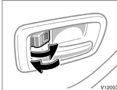
**LOCKING AND UNLOCKING WITH INSIDE LOCK KNOB**
