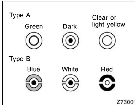
CHECKING BY HYDROMETER
