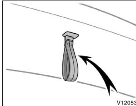
When closing the back door, use the inside strap for easier reach to the back door.
