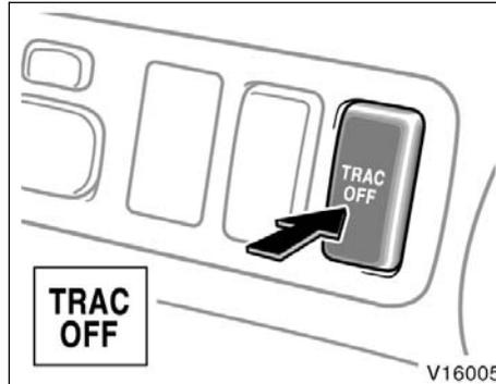
You can turn off the traction control system by pushing the "TRAC OFF" switch. The "TRAC OFF" indicator/warning light will come on. Pushing the "TRAC OFF" switch a second time turns on the traction control system again and the "TRAC OFF" indicator/warning light will go off. At this time, the vehicle skid control also turns off and on simultaneously.
