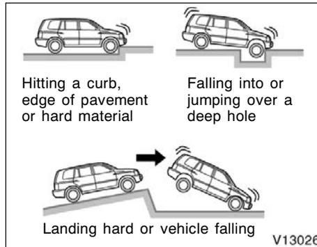
The SRS front airbags may deploy if a serious impact occurs to the underside of your vehicle. Some examples are shown in the illustration.
