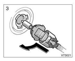
3. Insert the bulb base into the mounting hole by turning it clockwise.
