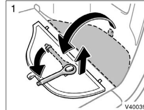
1. Pull up the deck board and remove the front towing eyelet by turning it counterclockwise. (For the towing eyelet location, see "—Required tools and spare tire" on page 215 in this section.)
