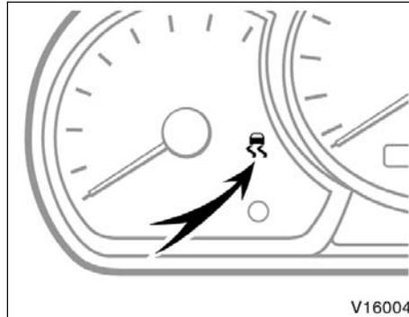
The traction control system automatically helps control the spinning of 4 wheels which may occur when accelerating on slippery road surfaces, thus assisting driver to control the driving power of 4 wheels.
