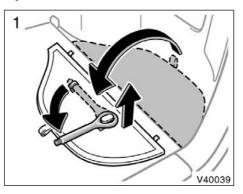
Pull up the deck board and remove the front towing eyelet by turning it counterclockwise. (For the towing eyelet location, see "—Required tools and spare tire" on page 215 in this section.)
