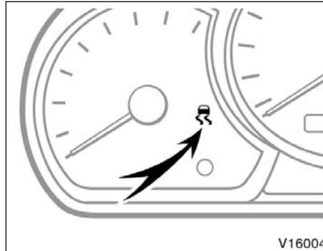
The vehicle skid control system helps integrated control of several systems such as an anti-lock brake system, brake assist system, traction control, engine control, etc. This system automatically controls the output of the brakes or engine to help prevent the vehicle from skidding when cornering on a slippery road surface or abrupt steering wheel operation occurs.
