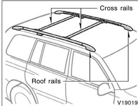
The roof luggage carrier consists of roof rails and sliding cross rails.
