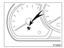
This SRS side airbag system has a service reminder indicator to inform the driver of operating problems. If either of the following conditions occurs, this indicates a malfunction of the airbags. Contact your Toyota dealer as soon as possible to service the vehicle.
