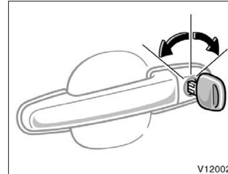
**LOCKING AND UNLOCKING WITH KEY**
