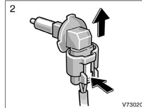
2. Pull the bulb out of the bulb base and install a new bulb.
