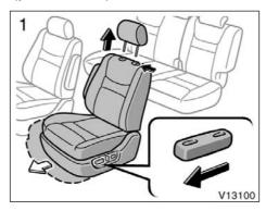
Remove the head restraint. Push the seat position adjusting switch forward to slide the seat further forward than the front-most lock position.
