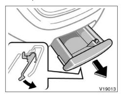
To use the box, pull out while holding the lever.
