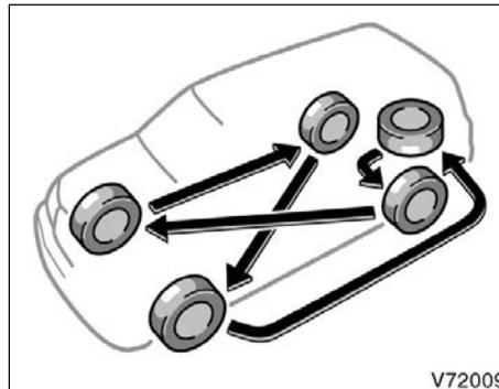
When rotating tires, check for uneven wear and damage. Abnormal wear is usually caused by incorrect tire pressure, improper wheel alignment, out-of-balance wheels, or severe braking.
