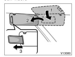
To block out glare, move the sun visor. To block out glare from the front—Swing down the sun visor (position 1).
