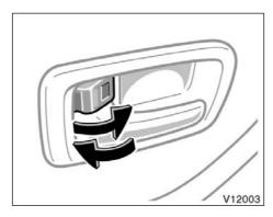
LOCKING AND UNLOCKING WITH INSIDE LOCK KNOB
