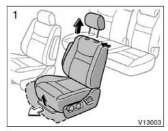
Remove the head restraint. Hold the center of the lever and pull it up. Then slide the seat further forward than the front-most lock position.
