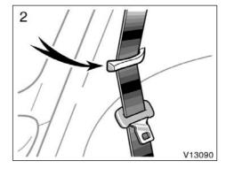
2. Make sure the outer seat belts passes through the hangers when folding the rear seat.
