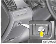
To open the trunk from inside the vehicle, press the trunk lid release button.
