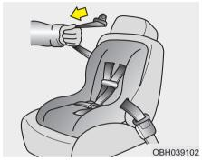
Pull the shoulder portion of the seat belt all the way out. When the shoulder portion of the seat belt is fully extended, it will shift the retractor to the "Aautomatic locking" (child restraint) mode.
