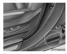
The vehicle certification label attached on the driver's side center pillar contains the vehicle identification number (VIN).
