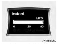
Instant fuel consumption (MPG or I/100km) This mode calculates the instant fuel consumption every 2 seconds (supervision type: every 0.2 second) from the driving distance and quantity of fuel
