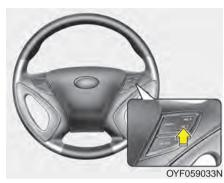
Push the SET- switch, and release it at the desired speed. The SET indicator light in the instrument cluster will illuminate. Release the accelerator at the same time. The desired speed will automatically be maintained.
