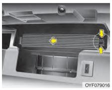
3. Remove the climate control air filter cover while pressing the lock on the right of the cover.
